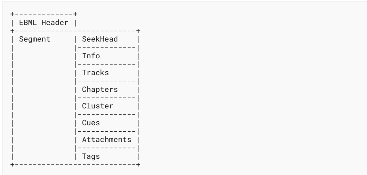
Figure 1: Basic Layout of a Matroska File
